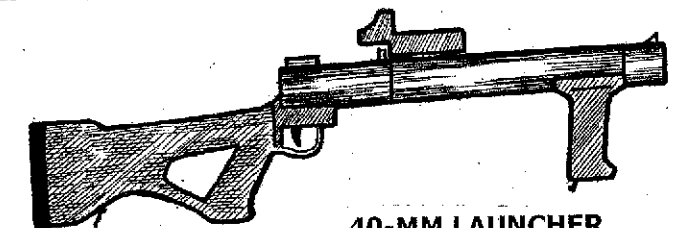
40-MM LAUNCHER Fires 40-mm rounds, single shot.
